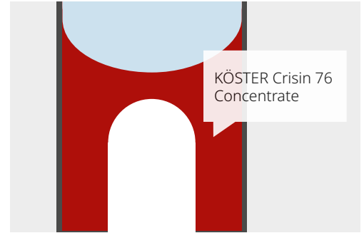
Narrowing/blocking the capillary, forming an elastic film in the capillary
