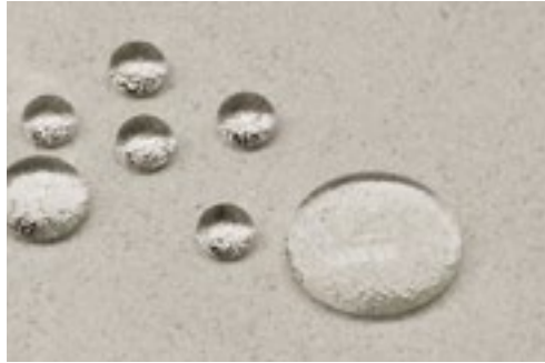
Hydrophobizing: Making the building material water repellent
